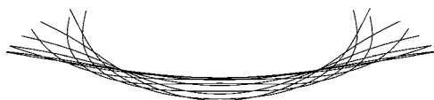
FIG. 15. Steady oscillation regime of the odd mode at Cm=25 , \omega=376.991 . Configurations for one period with time step 1/600 are shown.
